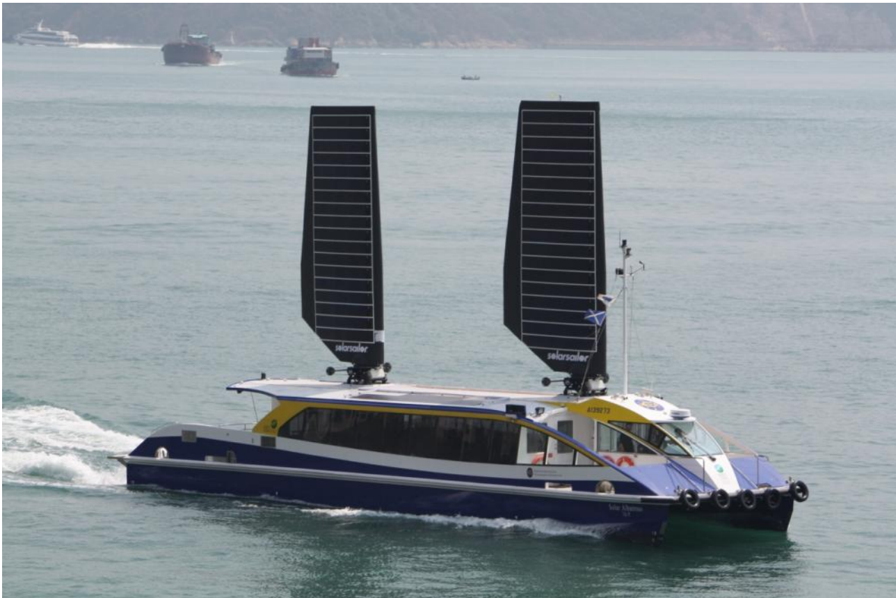
One of the new craft fitted with solar sails, recently delivered in Hong Kong *
